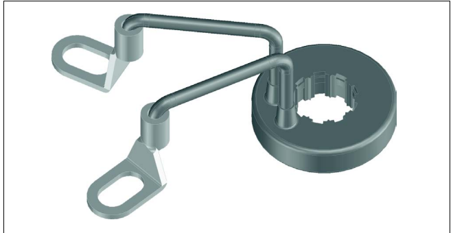
Fig. 6: Component for line break monitoring in conjunction with VEGATOR 632
