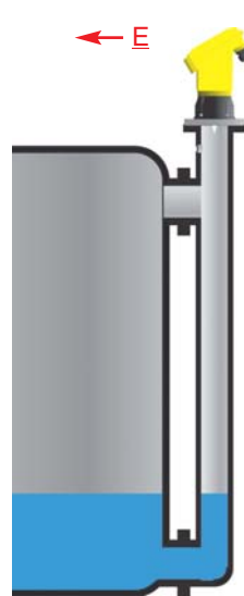
Fig 6.21 Bypass tube showing direction of polarization
