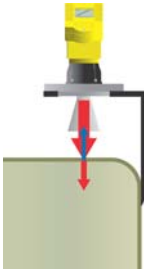
Fig 6.29 Flat plastic tank top gives a reflection directly back to the antenna
