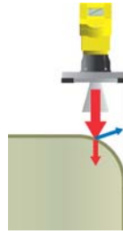
Fig 6.30 Angled plastic tank top improves the measurement of the liquid inside
