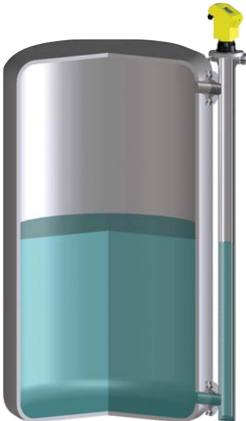
Fig 6.20 Stand pipe / stilling tube showing position of vent relative to polarization direction and overall length
