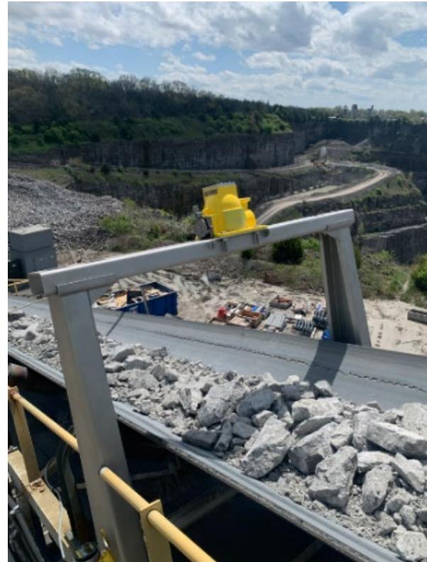
Calibration is a simple, two-step process: First, measure the count rate of the empty conveyor belt. Next, measure the count rate when the belt is loaded, then enter the product weight into the calibration table.
