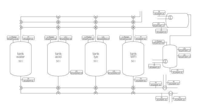
Schematic of a CIP system with level, pressure and point level sensors
