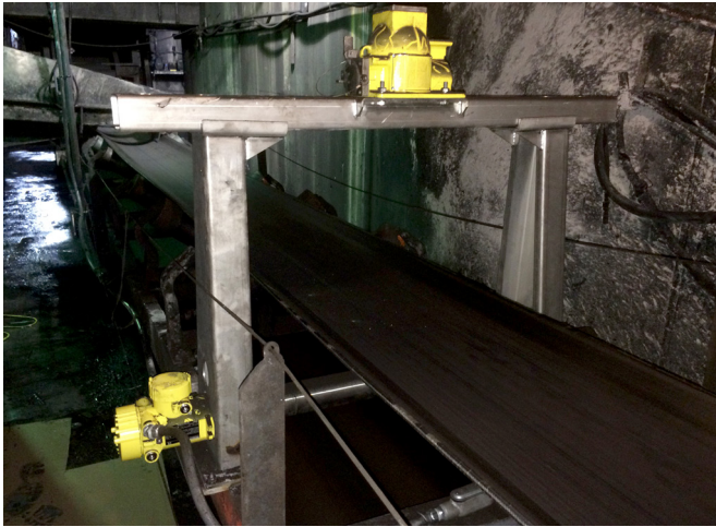
Figure 4. A mine replaced a load cell system with this radiometric material measurement system, resulting in a payback of eight months due to reduced required maintenance.
