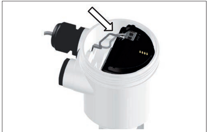
Fig. 3: Connection steps 5 and 6 - Single chamber housing
