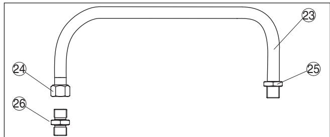
Fig. 9: Pre-assembled coolant hose
