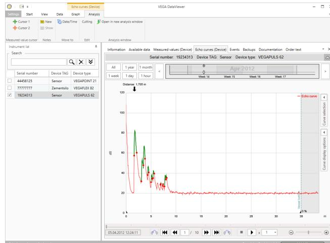
Fig. 8: Device data - Echo curve (DTM)
