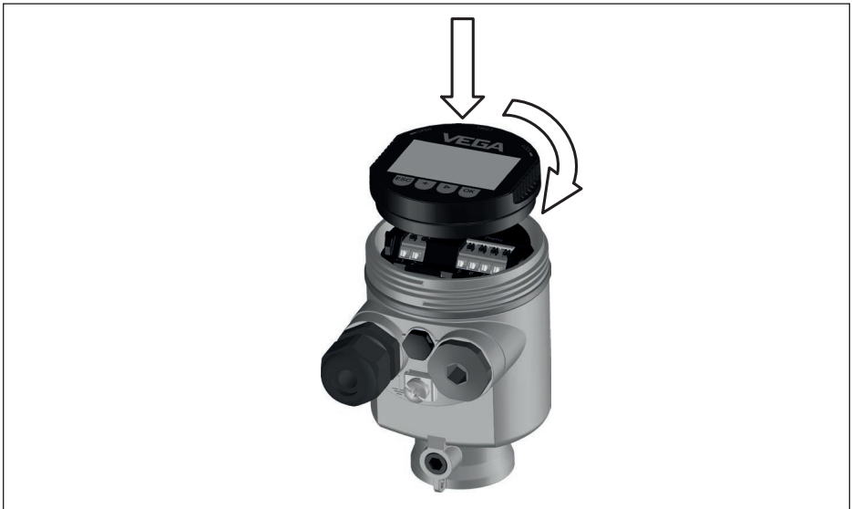
Fig. 1: Installing the display and adjustment module in the electronics compartment of the single chamber housing
