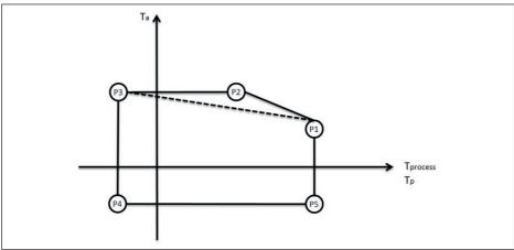
Furthermore it must be observed that the graph defined by the points P1 ... P5 was determined for instruments with a permissible process temperature of up to +195 °C with an isolation (heat conductance of 0.05 W/mK with 2 cm thick insulation). Two layers of insulation material with a thickness of 2 cm each were attached from the tank surface with the mentioned heat conductance.
