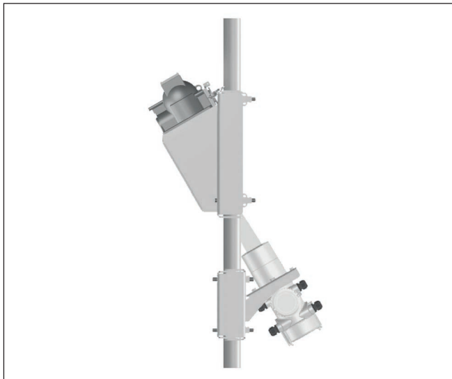
Fig. 11: 30° measurement setup on a pipeline with diameter 50 ... 100 mm (1.97 ... 3.94 in)
