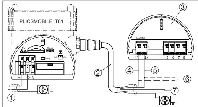
Fig. 6: Connection voltage supply and plics® sensor
