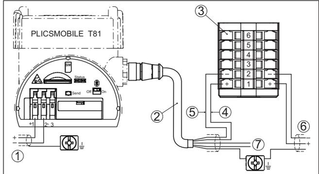
Fig. 7: Connection of the voltage supply and VEGABOX 03
