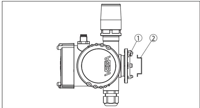
Fig. 3: PLICSMOBILE T81 for carrier rail mounting
