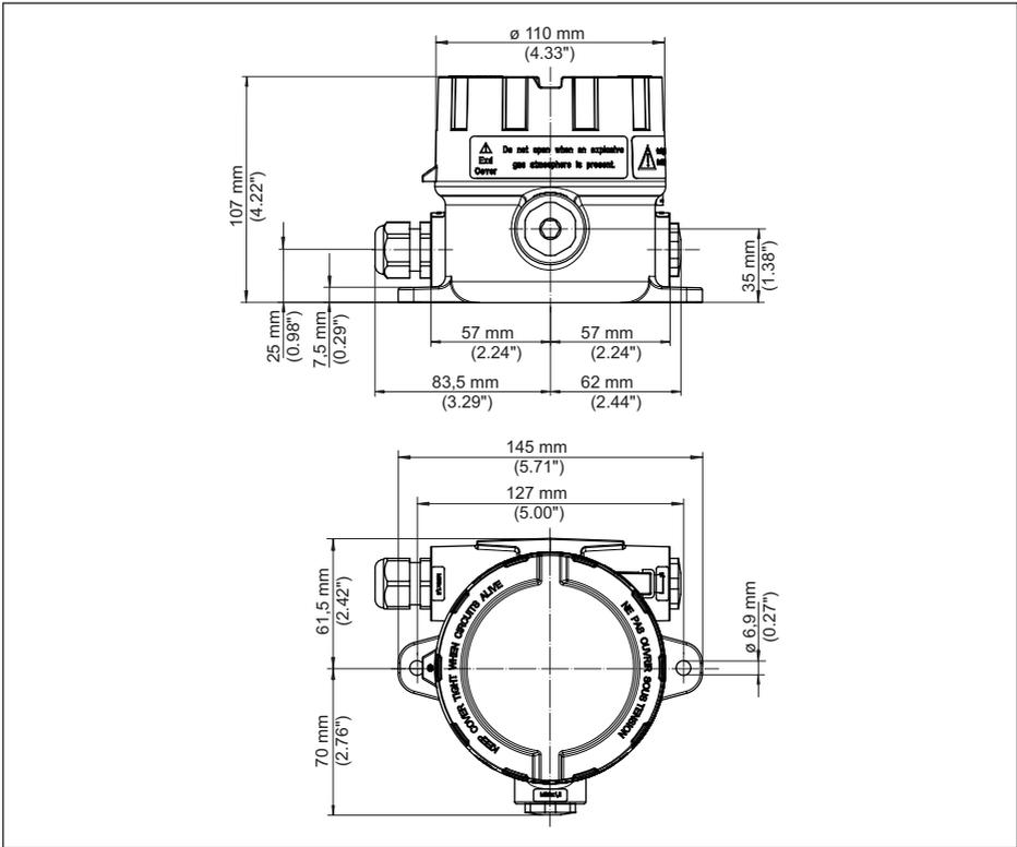
Fig. 21: Dimensions PLICSMOBILE B81 with Aluminium housing
