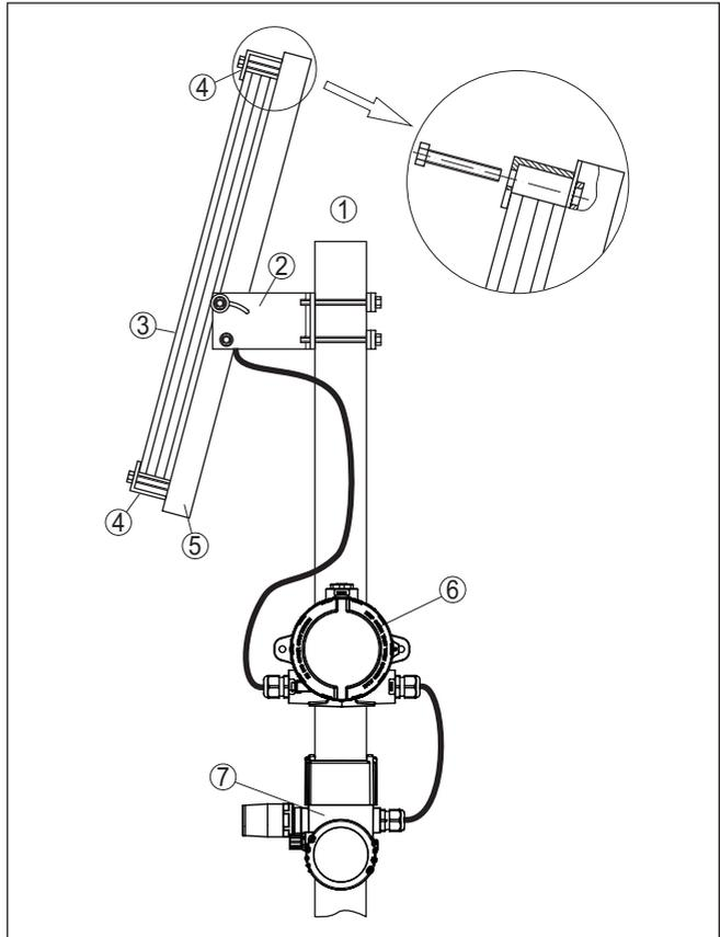
Fig. 13: Tube mounting PLICSMOBILE with solar module
