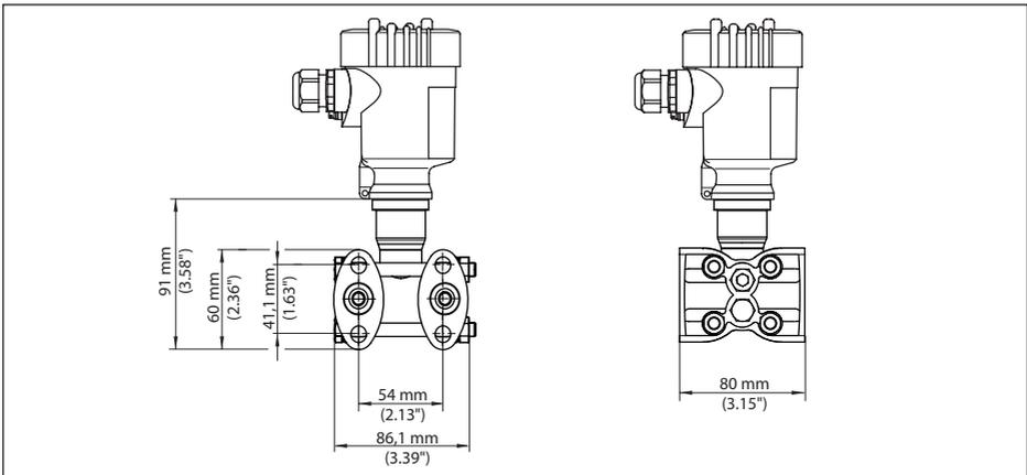
Fig. 47: VEGADIF 85, ¼-18 NPT connection, with lateral ventilation
