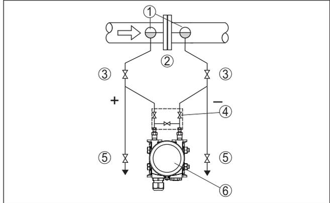
Fig. 18: Measurement setup, flow measurement in vapours
