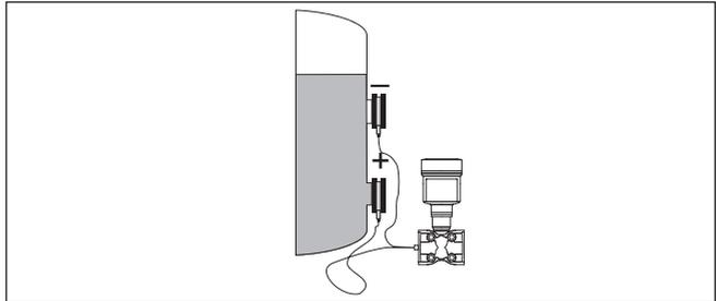
Fig. 5: Density measurement with VEGADIF 85
