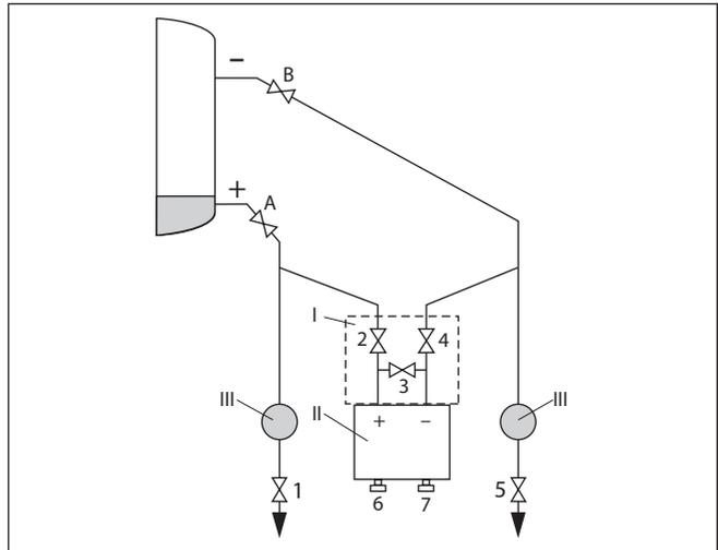
Fig. 36: Preferred measurement setup for closed vessels
