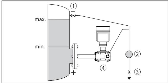
Fig. 14: Measurement setup, level measurement in closed vessel
