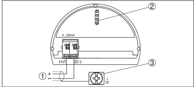
Fig. 31: Electronics and connection compartment - single chamber housing
