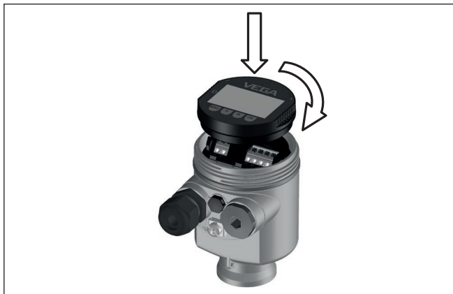
Fig. 36: Installing the display and adjustment module in the electronics compartment of the single chamber housing
