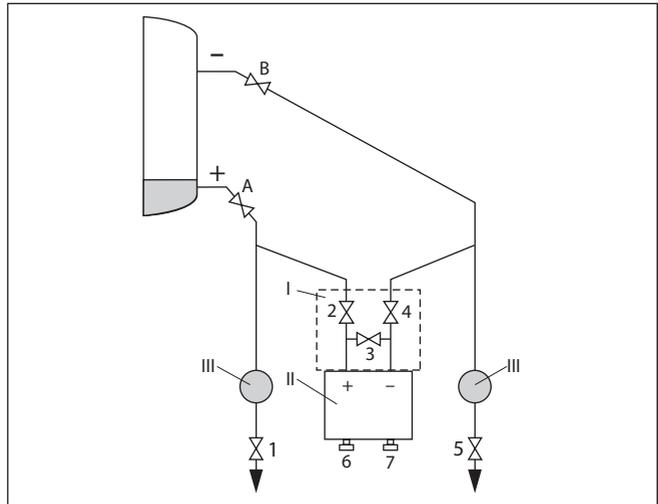
Fig. 43: Preferred measurement setup for closed vessels
