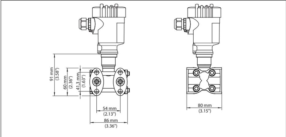
Fig. 51: VEGADIF 85, ventilation on process axis
