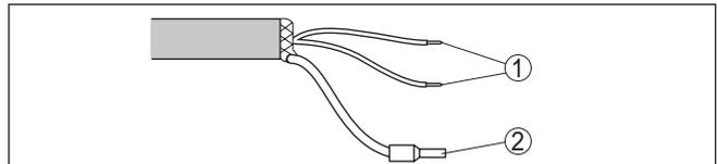
Fig. 31: Wire assignment in permanently connected connection cable
