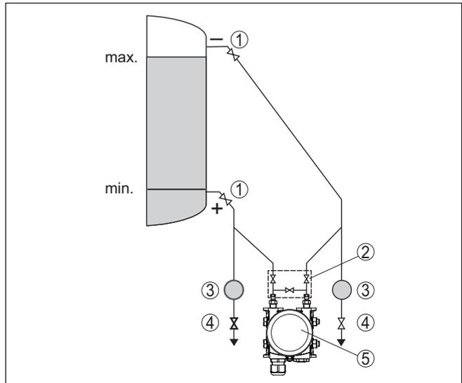
Fig. 12: Measurement setup, level measurement in closed vessel
