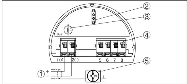
Fig. 34: Electronics and connection compartment - single chamber housing
