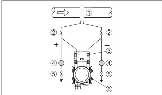
Fig. 18: Measurement setup, flow measurement in liquids
