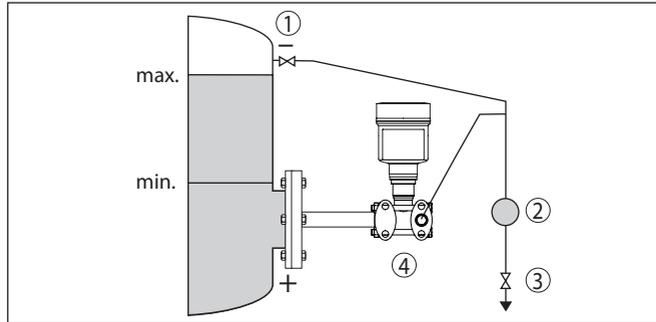
Fig. 13: Measurement setup, level measurement in closed vessel
