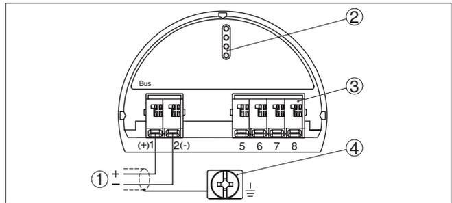
Fig. 30: Connection compartment - double chamber housing
