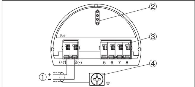
Fig. 28: Connection compartment - double chamber housing
