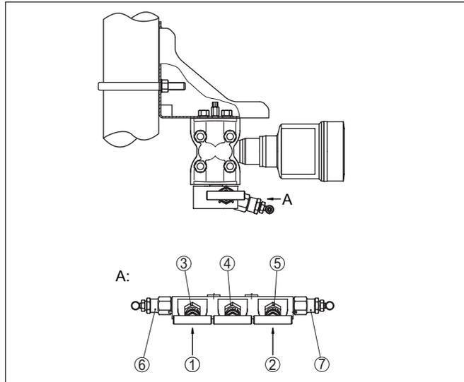
Fig. 11: Connection of a 5-fold valve block
