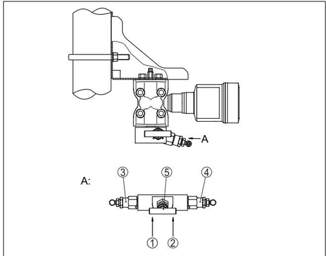
Fig. 9: Connection of a 3-fold valve block
