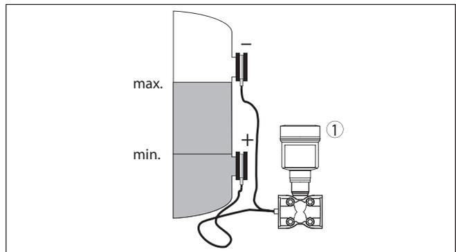
Fig. 14: Measurement setup, level measurement in closed vessel
