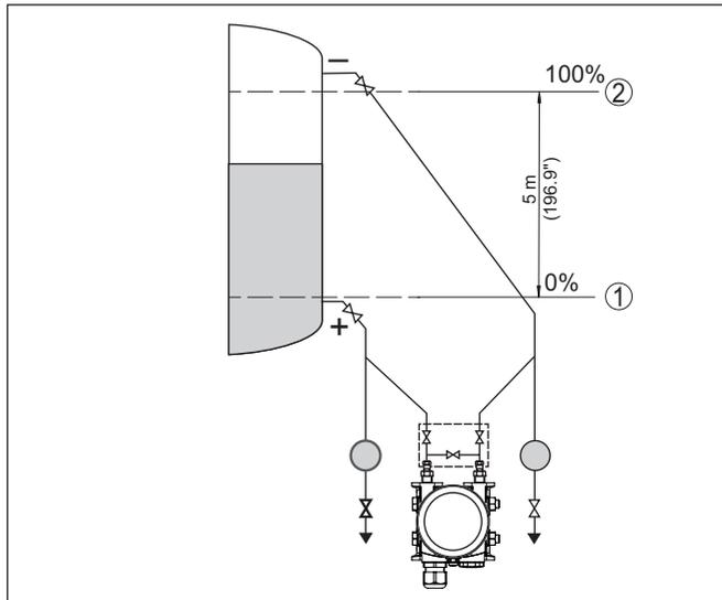
Fig. 40: Parameter adjustment example Min./max. adjustment, level measurement
