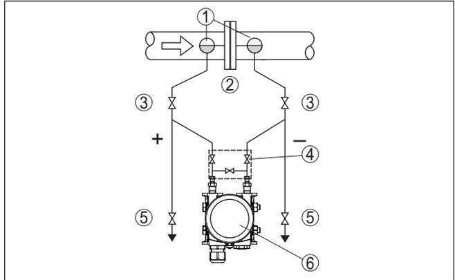
Fig. 17: Measurement setup, flow measurement in vapours
