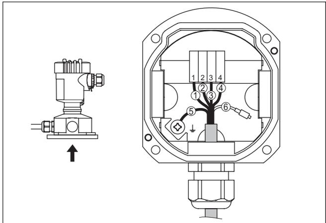
Fig. 33: Connection of the process component in the housing base
