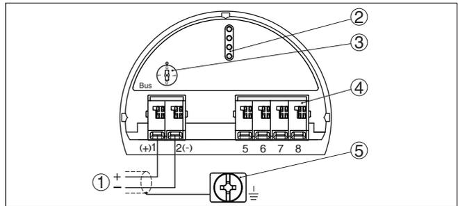
Fig. 26: Electronics and connection compartment - single chamber housing
