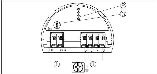
Fig. 27: Electronics compartment - double chamber housing
