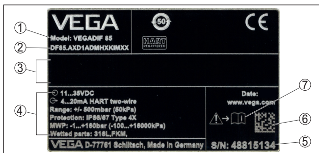
Fig. 1: Layout of the type label (example)
