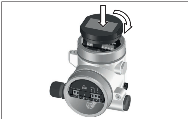
Fig. 33: Insertion of the display and adjustment module
