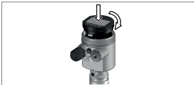
Fig. 11: Installing the display and adjustment module in the electronics compartment of the single chamber housing
