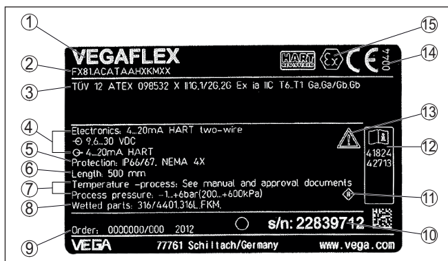
Fig. 1: Layout of the type label (example)
