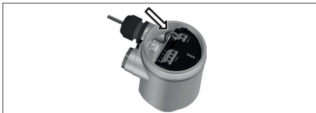
Fig. 7: Connection steps 5 and 6 - Single chamber housing
