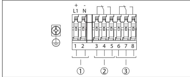
Fig. 13: Wiring plan, single chamber housing
