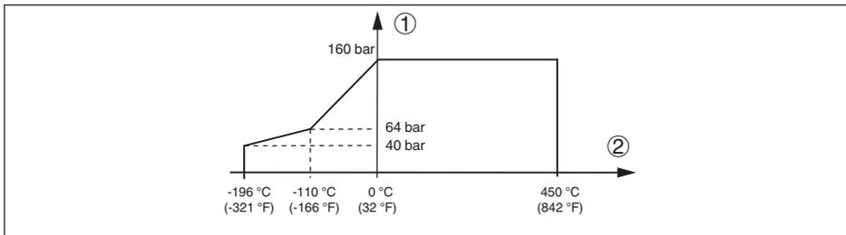
Fig. 18: Process temperature - Process pressure - Version up to 160 bar (2321 psig)
