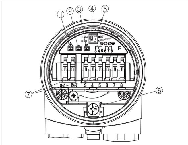
Fig. 12: Electronics and connection compartment, single chamber housing
