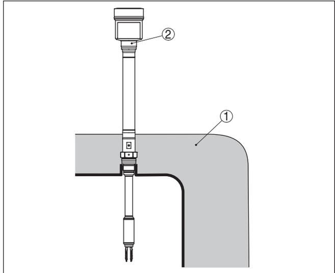
Fig. 8: Mounting the instrument on insulated vessels.
