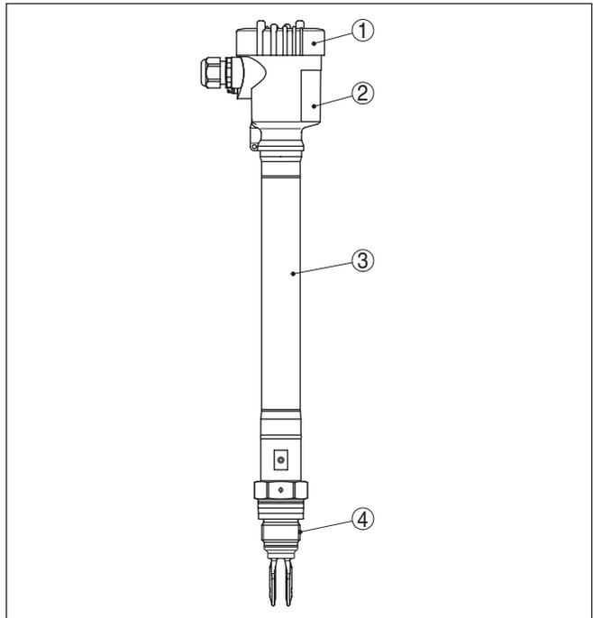
Fig. 1: VEGASWING 66 - compact version with plastic housing
