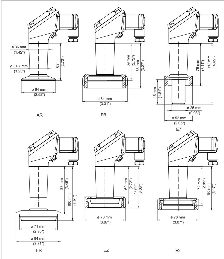
Fig. 41: VEGABAR 38, hygienic fitting
