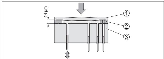
Fig. 4: Configuration of the Mini-CERTEC® measuring cell
