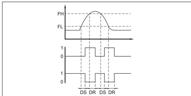
Fig. 27: Effect of the delay time on the output with window function
