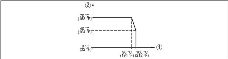
Fig. 36: Temperature derating VEGABAR 38, with activated Bluetooth communication
