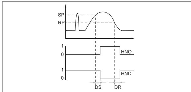
Fig. 26: Effect of the delay time on the output with hysteresis function
