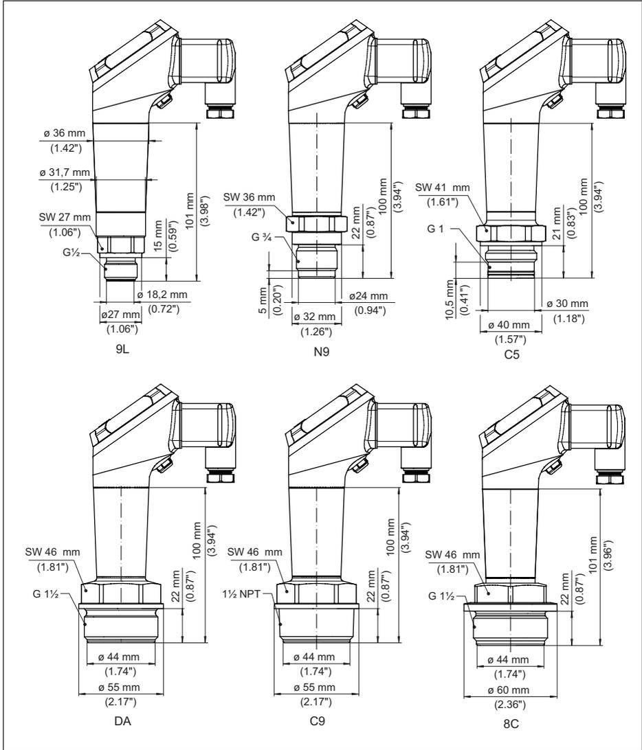
Fig. 39: VEGABAR 38, threaded fitting front-flush
