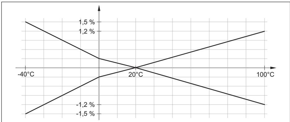
Fig. 34: Temperature error with TD 1 : 1
