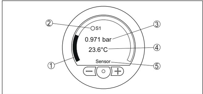
Fig. 22: Measured value, switching status and additional data (example electronics A and C)
