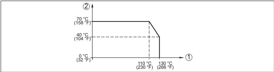
Fig. 35: Temperature derating VEGABAR 38
