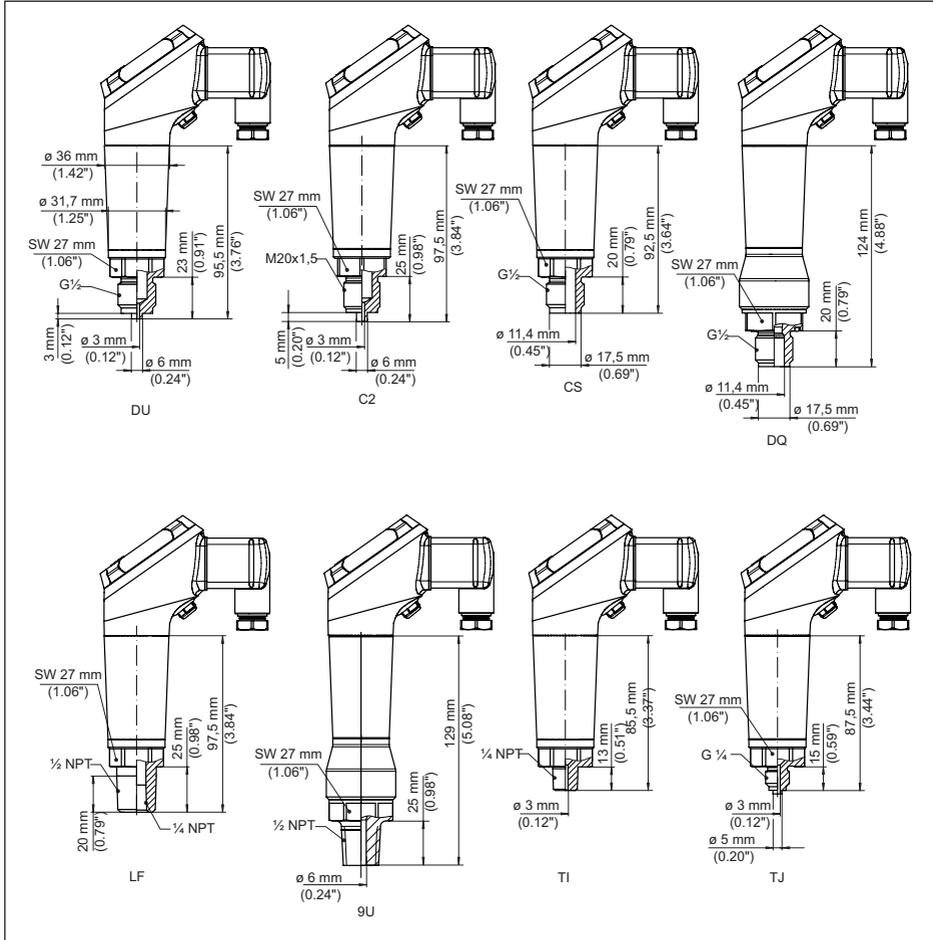
Fig. 38: VEGABAR 38, threaded fitting not front-flush
