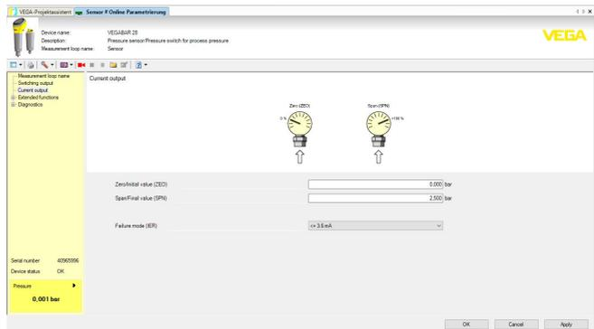
Fig. 31: Example of a DTM view - Adjustment current output
