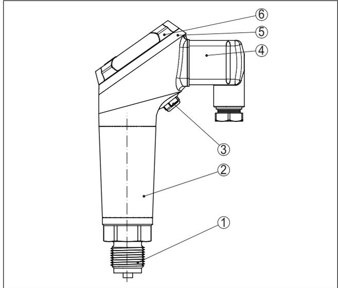
Fig. 1: Components of VEGABAR 38
