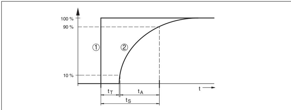
Fig. 33: Behaviour the current output in case of sudden change of the process variable.  $t_T$ : dead time;  $t_A$ : rise time;  $t_S$ : jump response time
