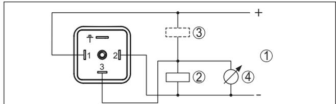
Fig. 20: Wiring plan - Three-wire 1 x transistor or 4 ... 20 mA
