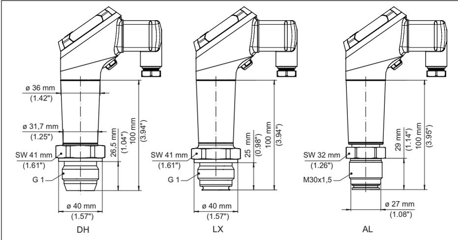
Fig. 40: VEGABAR 38, cone/extension fitting
