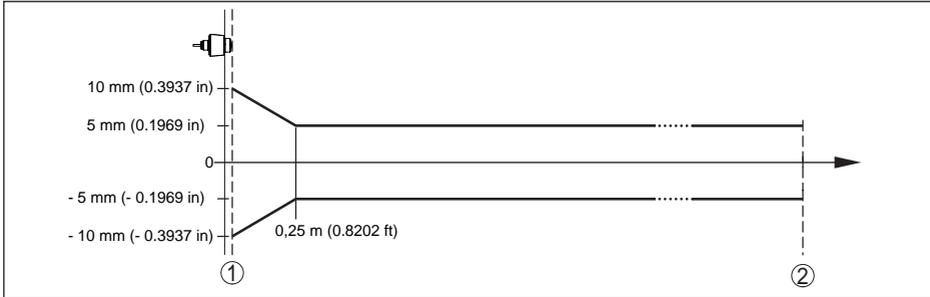
Fig. 24: Deviation under reference conditions <sup>9)</sup>
