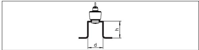
Fig. 11: Socket mounting with deviating socket dimensions
