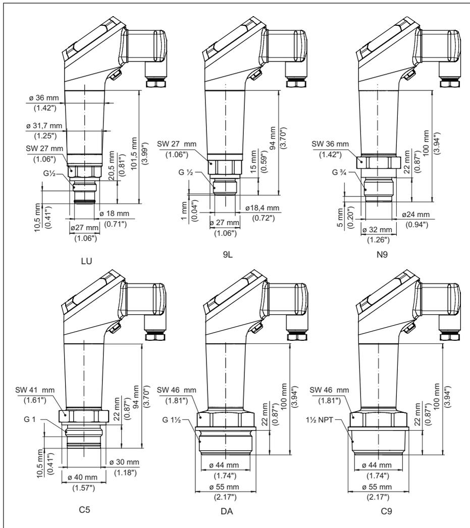
Fig. 36: VEGABAR 39, raccord fileté arasant
