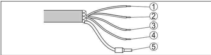
Fig. 17: Wire assignment in permanently connected connection cable
