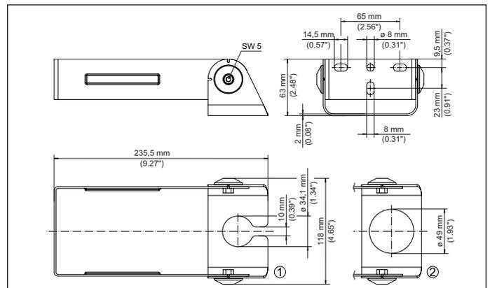
Fig. 26: Mounting strap for wall mounting - bracket 200 mm
