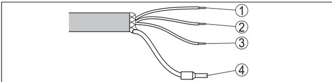
Fig. 16: Wire assignment in permanently connected connection cable
