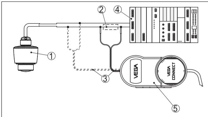
Fig. 19: Connecting the PC to the signal cable
