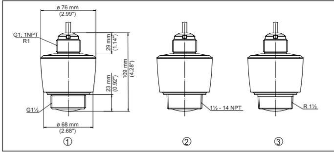
Fig. 21: Dimensions VEGAPULS C 11, C 21
