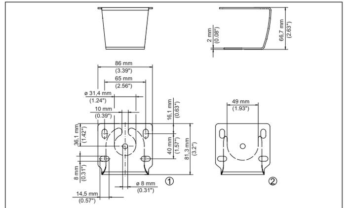
Fig. 25: Mounting strap for ceiling mounting
