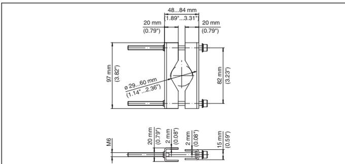
Fig. 14: Dimensions Brackets for tube mounting VEGAMET 841, 842
