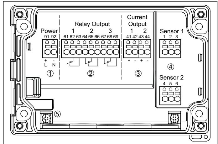
Fig. 7: Wiring plan VEGAMET
