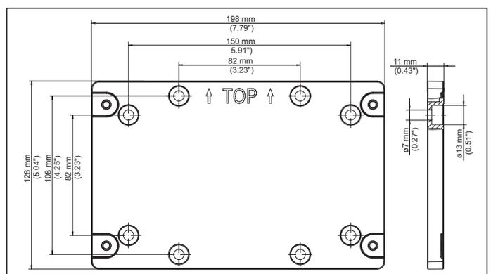
Fig. 16: Dimensions Wall mounting VEGAMET 861, 862
