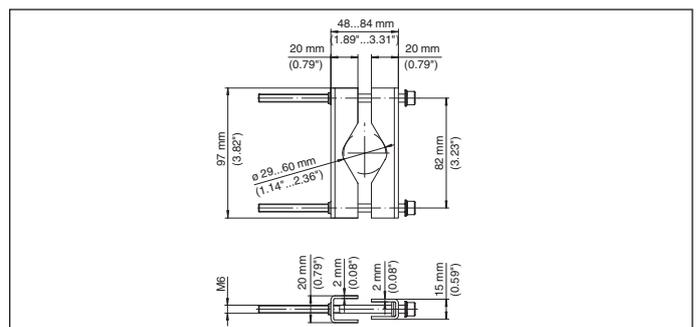
Fig. 18: Dimensions Brackets for tube mounting VEGAMET 861, 862
