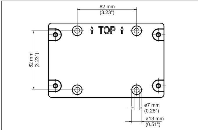
Fig. 2: Mounting plate for wall mounting (VEGAMET 841, 842)
