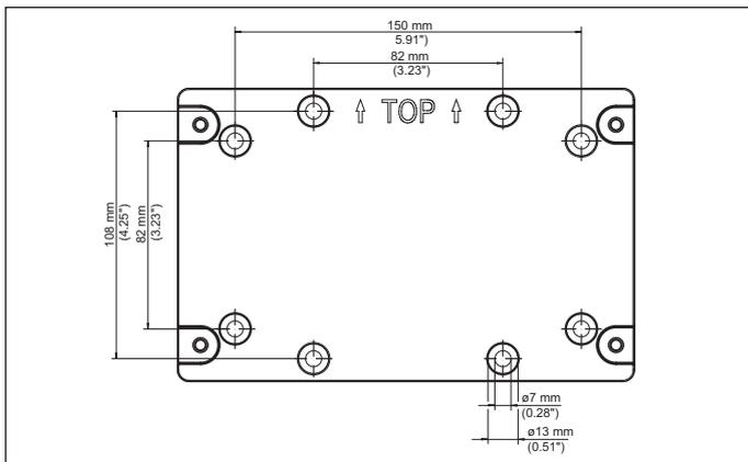
Fig. 3: Mounting plate for wall mounting (VEGAMET 861, 862)
