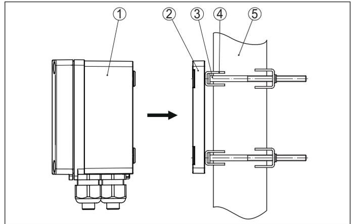
Fig. 4: Tube mounting
