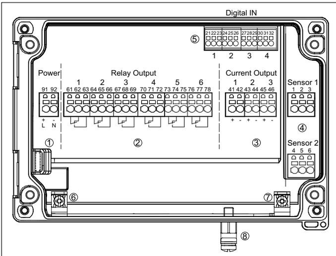
Fig. 9: Wiring plan VEGAMET
