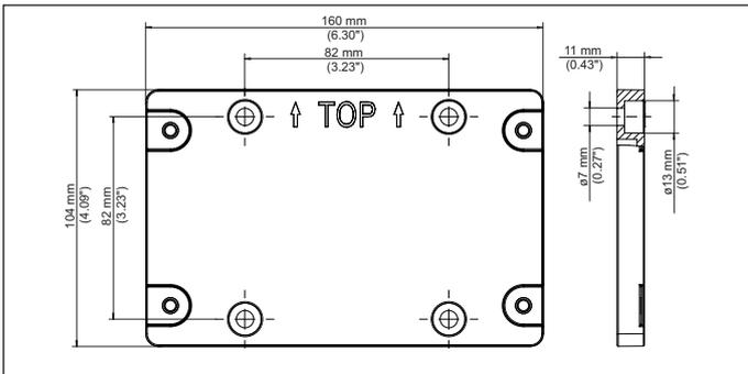
Fig. 12: Dimensions Wall mounting VEGAMET 841, 842
