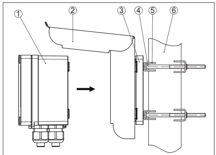
Fig. 5: Mounting sun protection with pipe mounting
