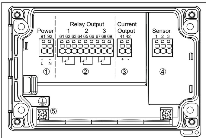
Fig. 6: Wiring plan VEGAMET
