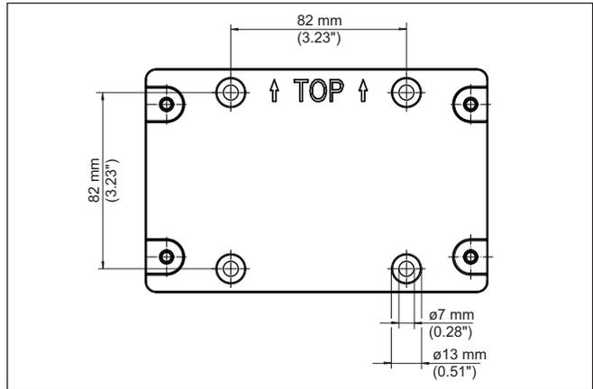
Fig. 3: Mounting plate for wall mounting VEGAMET 842
