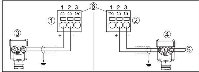
Fig. 7: Sensor input 1 for two-wire/four-wire sensor (active/passive)
