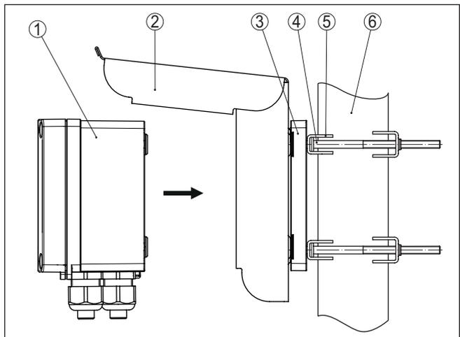
Fig. 5: Mounting sun protection with pipe mounting
