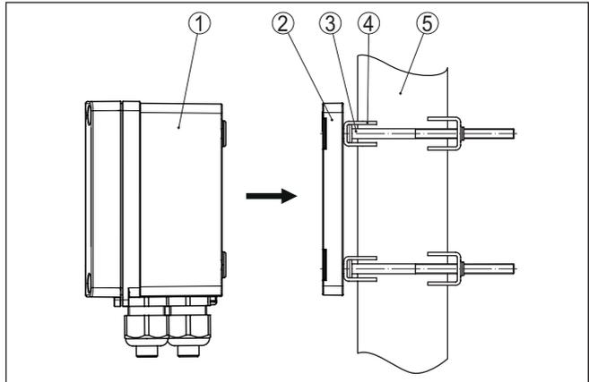
Fig. 4: Tube mounting
