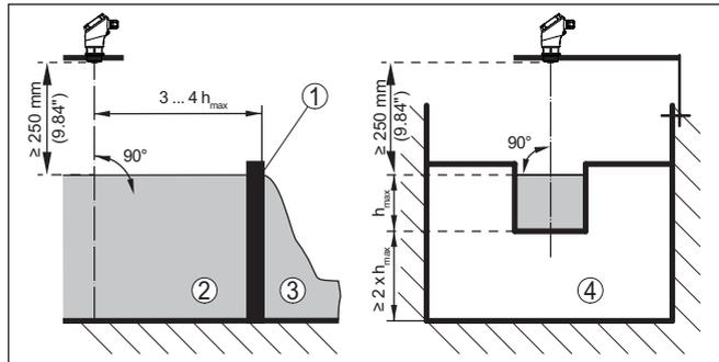
Fig. 22: Flow measurement with rectangular flume:  $h_{\text{max}} = \text{max. filling of the rectangular flume}$
