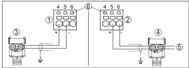
Fig. 8: Sensor input 2 for two-wire/four-wire sensor (active/passive)
