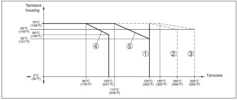
1 Version: METEC measuring cell, process temperature max. 150 °C
