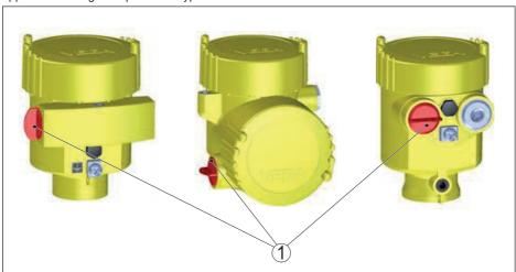
1 Red thread or dust cover must be removed before setup. The opening must be closed before setup by a way approved for the ignition protection type.
