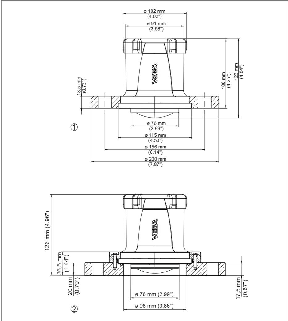
Fig. 22: Dimensions VEGAPULS Air 42
