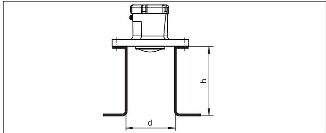
Fig. 9: Socket mounting with deviating socket dimensions
