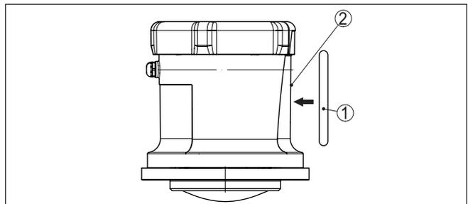
Fig. 13: Sensor activation via NFC technology
