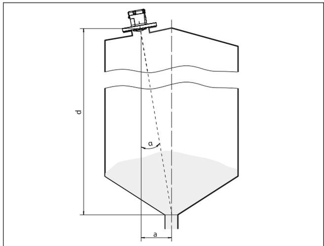
Fig. 12: Proposal for installation after orientation VEGAPULS Air 42
