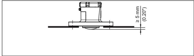
Fig. 8: Recommended socket mounting of VEGAPULS Air 42
