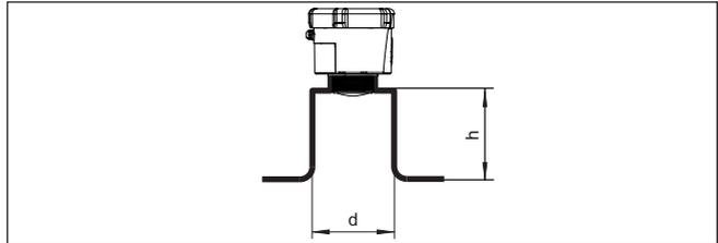
Fig. 9: Socket mounting with deviating socket dimensions
