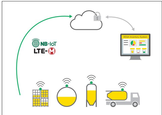
Fig. 2: Wireless measured value transmission via mobile radio
