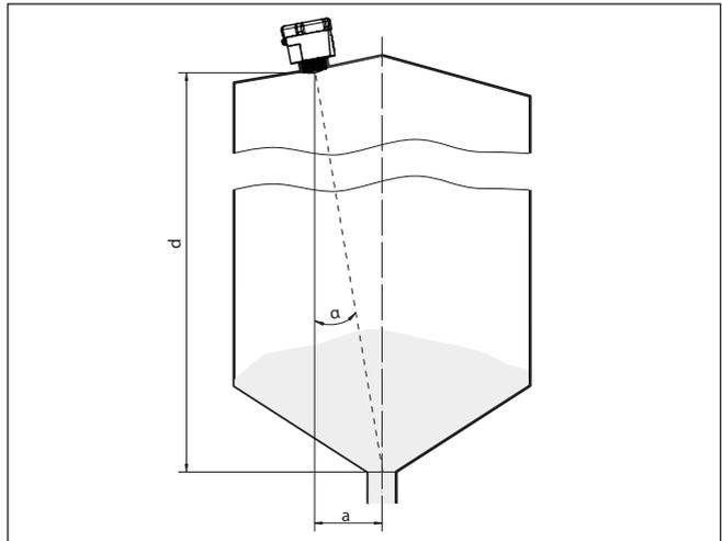
Fig. 12: Proposal for installation after orientation VEGAPULS Air 41
