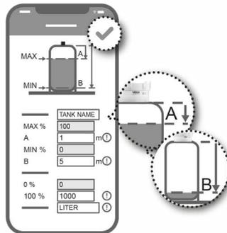
The onboarding of the sensor is completed. The VEGAPULS Air 41 is integrated in the VEGA Inventory System.
