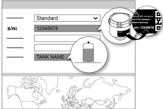
7. Open "**Configuration - Adjustment/Linearization**" and assign a linearization to VEGAPULS Air 41.
