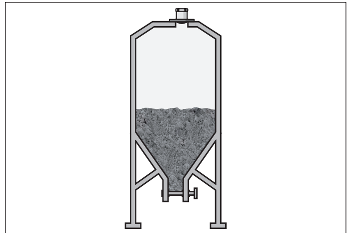
Fig. 15: Level measurement VEGAPULS Air 42 in the building material silo
