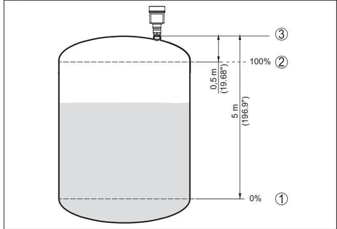
Fig. 9: Parameterisation example min./max. adjustment - liquids
