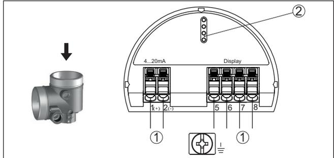
Fig. 6: Electronics compartment - double chamber housing
