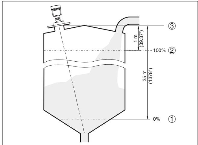
Fig. 10: Parameterisation example min./max. adjustment - bulk solids
