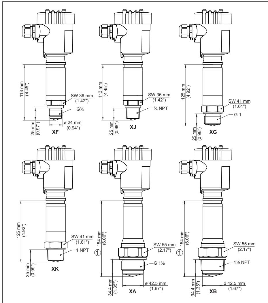
插图. 98: VEGAPULS 6X, 带有内置天线系统的螺纹至 +200 °C (+392 °F)/+250 °C (+482 °F)
