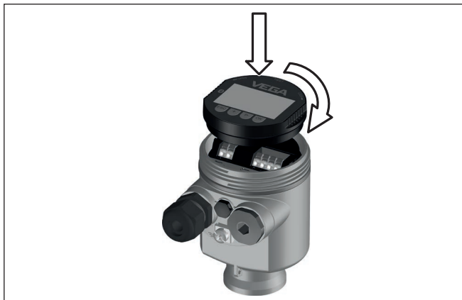
Fig. 49: Installing the display and adjustment module in the electronics compartment of the single chamber housing
