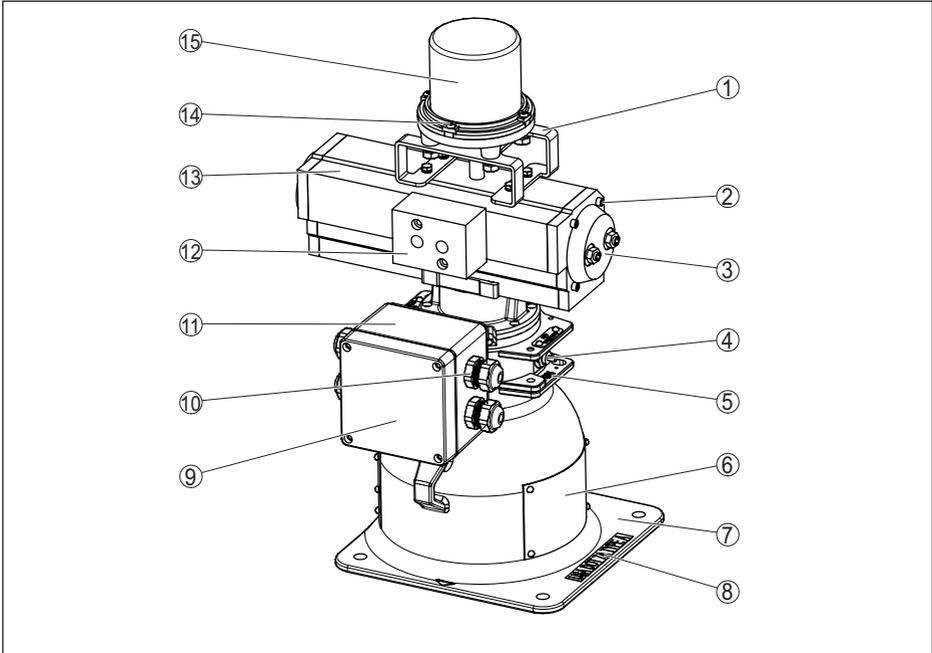
Fig. 35: Materials VEGASOURCE 82 - Version B - with ON/OFF position switches
