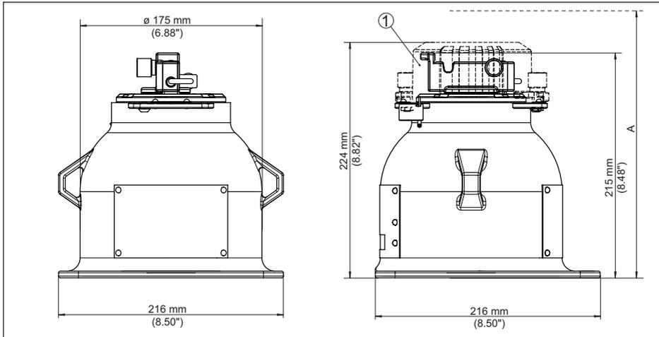
Fig. 37: Source holder VEGASOURCE 82, version X, C - Manual changeover
