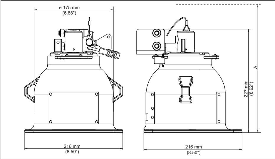
Fig. 39: Source holder VEGASOURCE 82, version X, C - Manual switchover with Interlock switch
