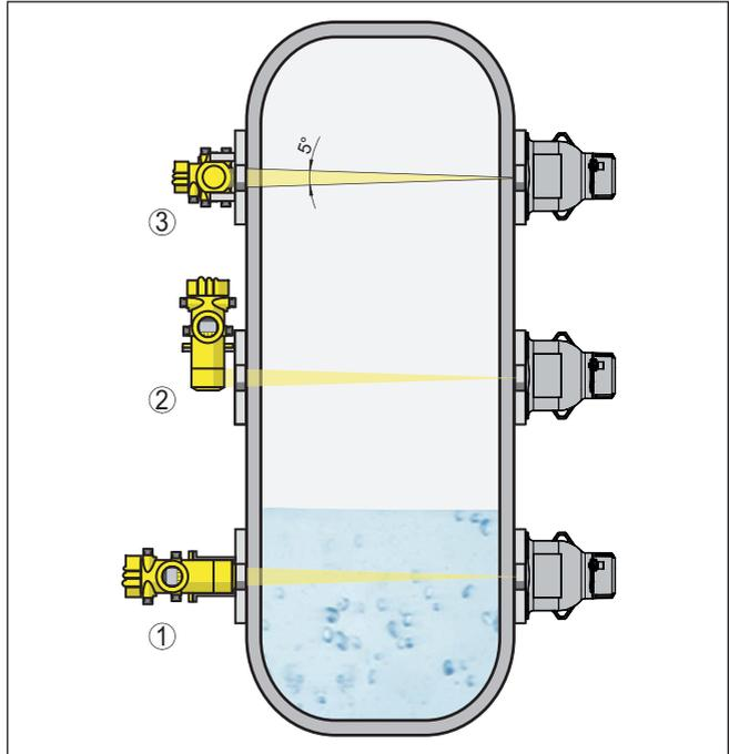
Fig. 13: Installation positions - Point level detection with MINITRAC 31
