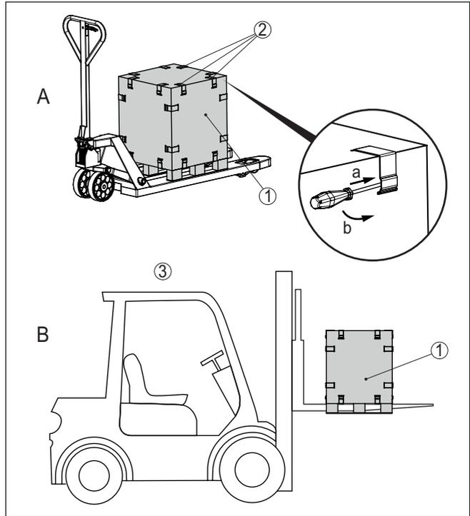
Fig. 7: Pallet transport of the type A packaging
