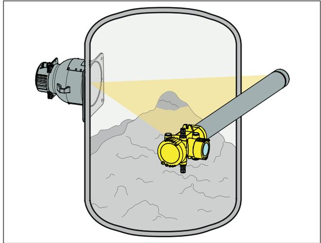
Fig. 14: Point Level detection with SOLITRAC 31
