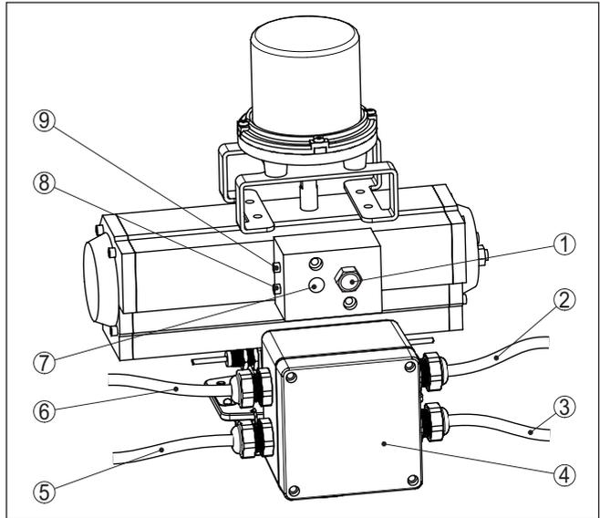
Fig. 22: Connection of the pneumatic lines on VEGASOURCE 82 - version B
