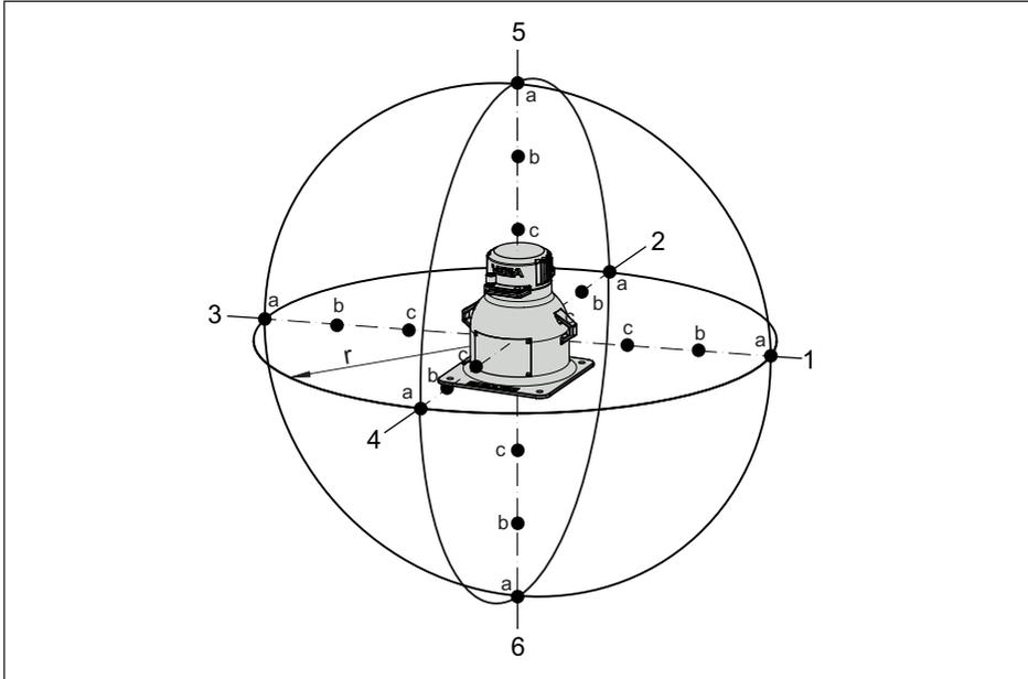
Fig. 36: Dose rate diagram (distance: 1 m) - example: source holder VEGASOURCE 82 with Cs-137, 200 mCi (7.4 GBq)
