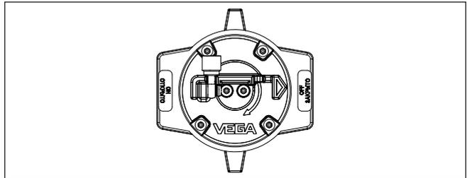
Fig. 26: Radiation OFF - VEGASOURCE 82 Version X, C
