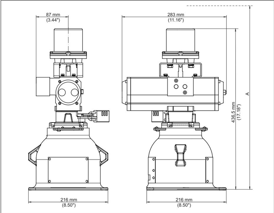
Fig. 40: Source holder VEGASOURCE 82, version B - Pneumatic switching
