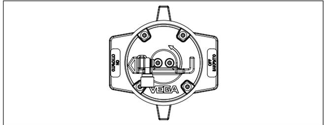
Fig. 25: Radiation ON - VEGASOURCE 82 Version X, C
