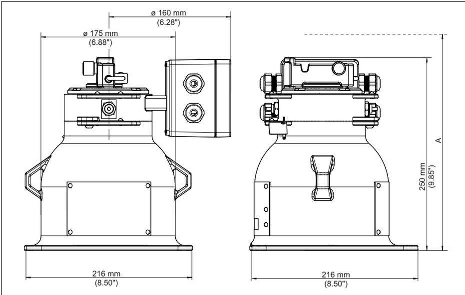
Fig. 38: Source holder VEGASOURCE 82, version X, C - Manual switchover with ON/OFF position switches
