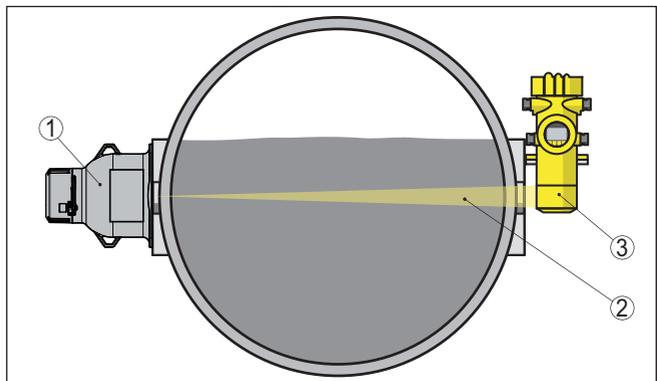
Fig. 18: Measurement setup on a horizontal pipeline
