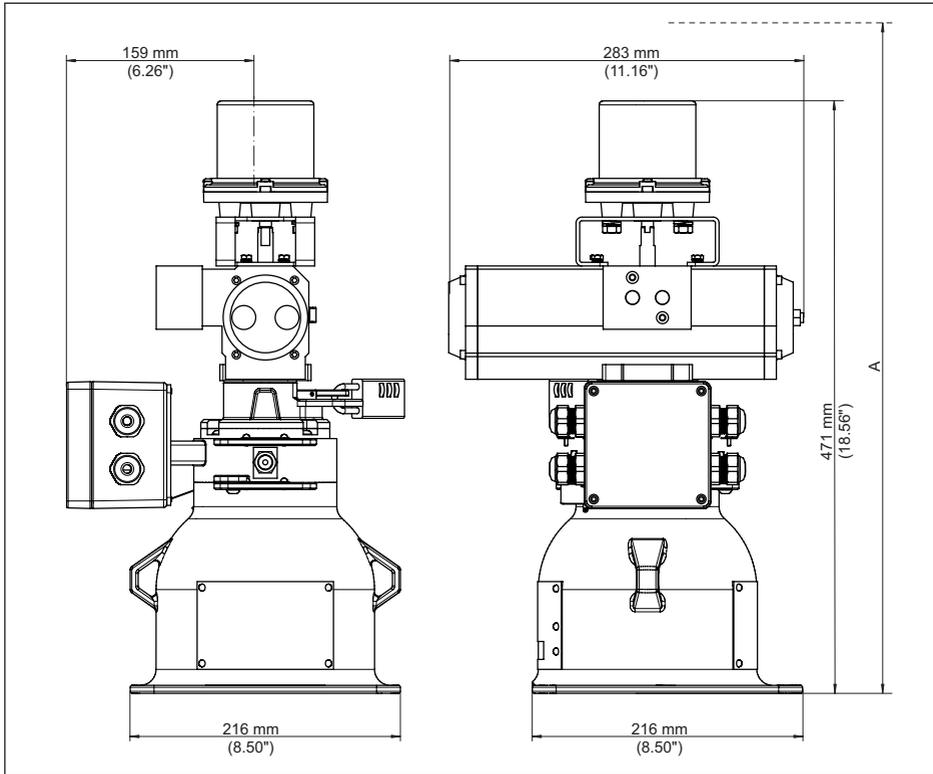
Fig. 41: Source holder VEGASOURCE 82, version B - Pneumatic switchover with ON/OFF position switches
