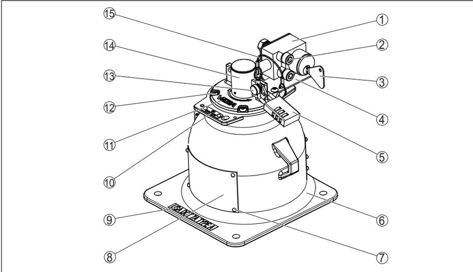
Fig. 33: Materials VEGASOURCE 82 - Version X, C - with Interlock switch
