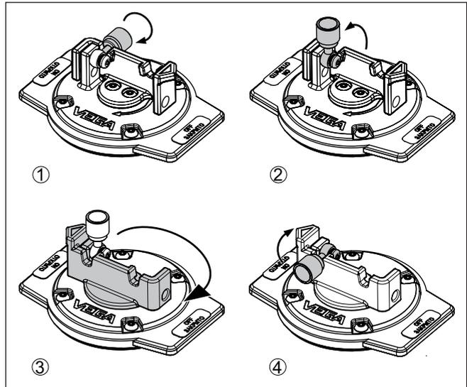
Fig. 24: Switching the radiation on - VEGASOURCE 82 version X, C
