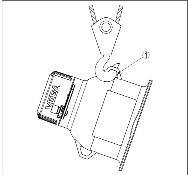
Fig. 9: Crane transport of the source holder
