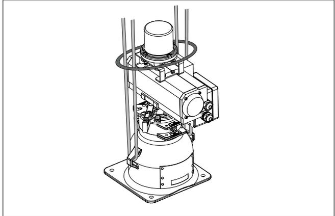
*Fig. 8: Lifting of a source holder with pneumatic switchover*
