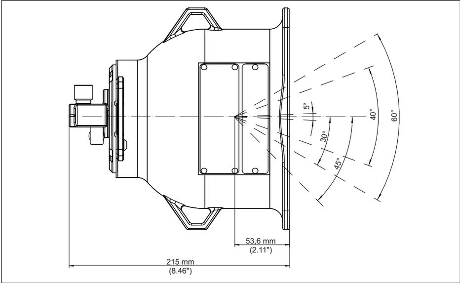
Fig. 42: Beam exit channel (e.g. version X, C)
