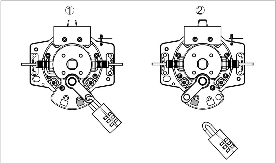
Fig. 28: Indication of the switching status with VEGASOURCE 82 - Version B - Pneumatic switchover
