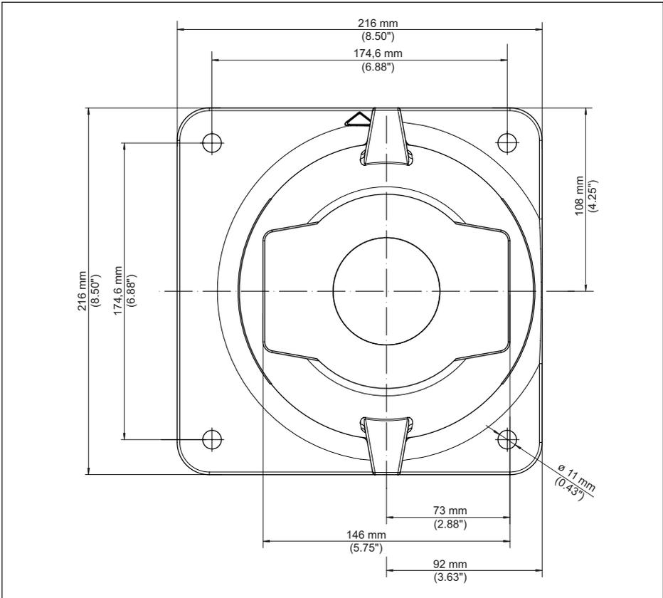
Fig. 43: Base plate with holes (e.g. version X, C)
