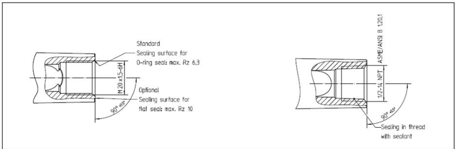
**Stainless-steel housing (fine cast) with M20 x 1.5 thread, ½ NPT thread**
