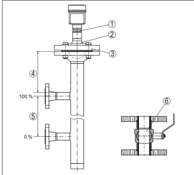
Fig. 41: Structure du tube bypass
