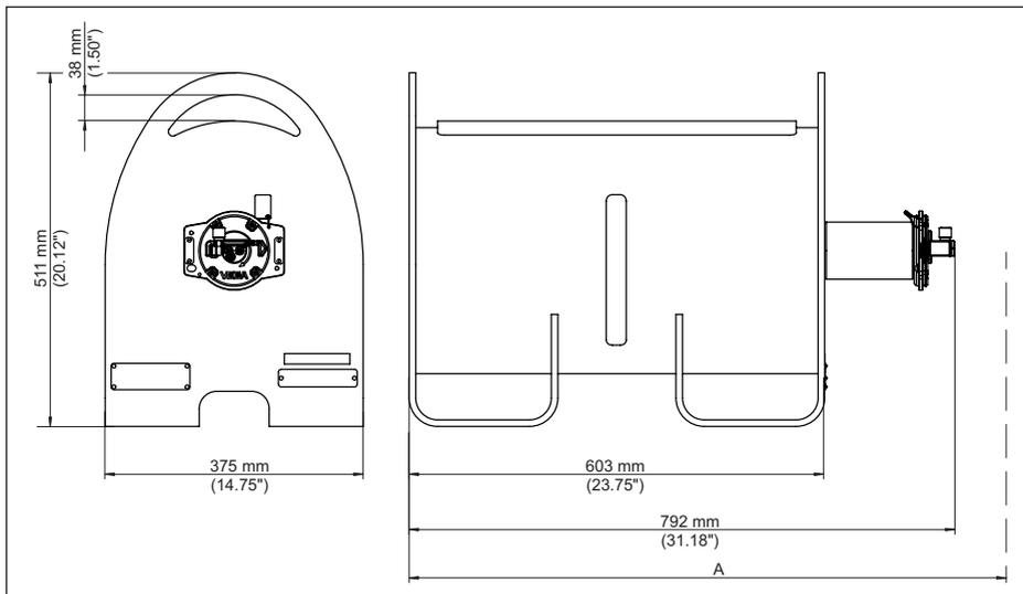
Fig. 24: Conteneur blindé VEGASOURCE 85, version X, C - commutation MARCHE/ARRÊT manuelle
