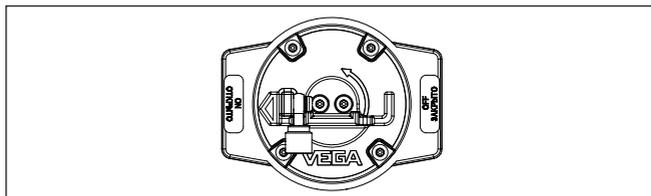
Fig. 17: Rayonnement "ON" - VEGASOURCE 85 Version X, C
