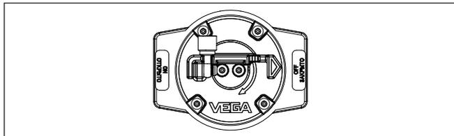
Fig. 18: Rayonnement "OFF" - VEGASOURCE 85 Version X, C
