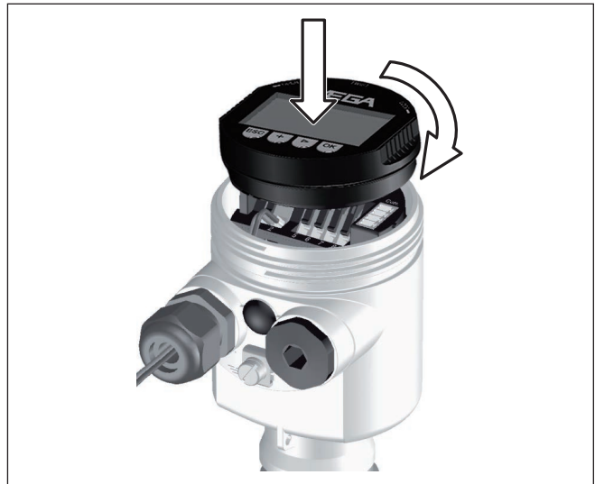
Fig. 21: Insert display and adjustment module in the single chamber housing
