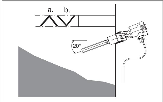
Fig. 3: Horizontal installation
