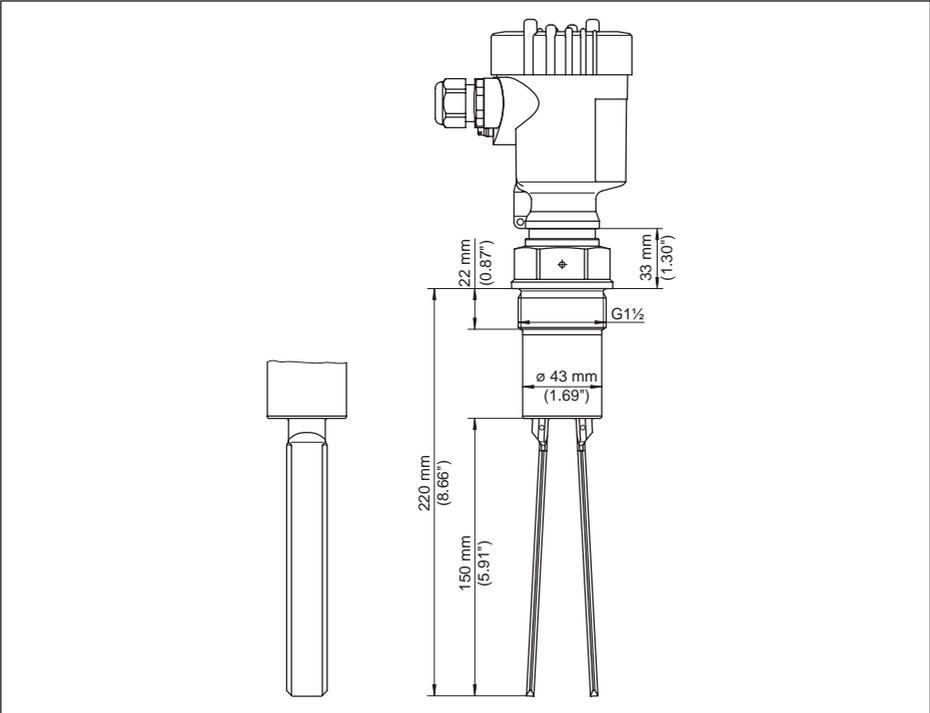
Fig. 32: VEGAWAVE 61, threaded version G1½ (DIN ISO 228/1)
