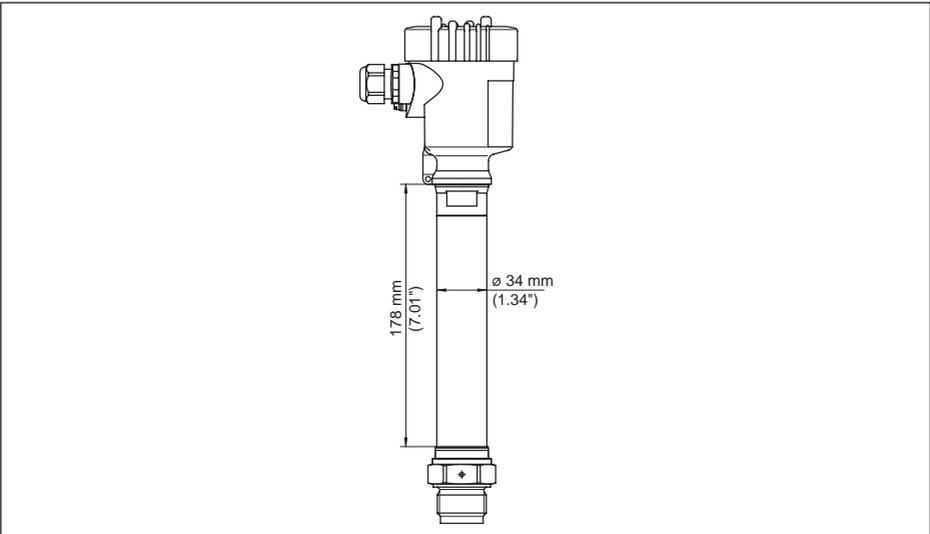
Fig. 33: Temperature adapter
