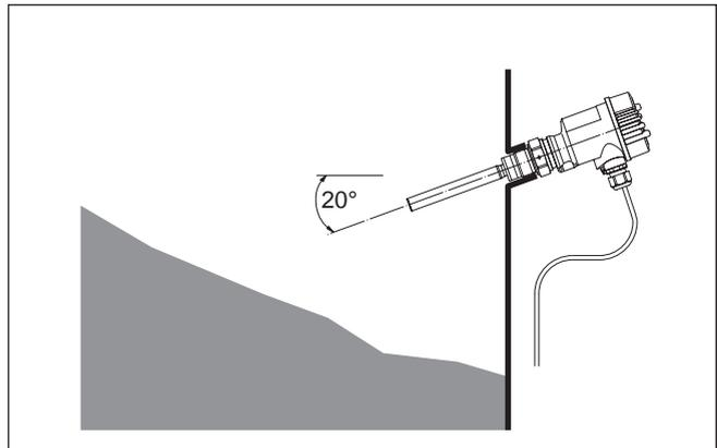
Fig. 4: Horizontal mounting
