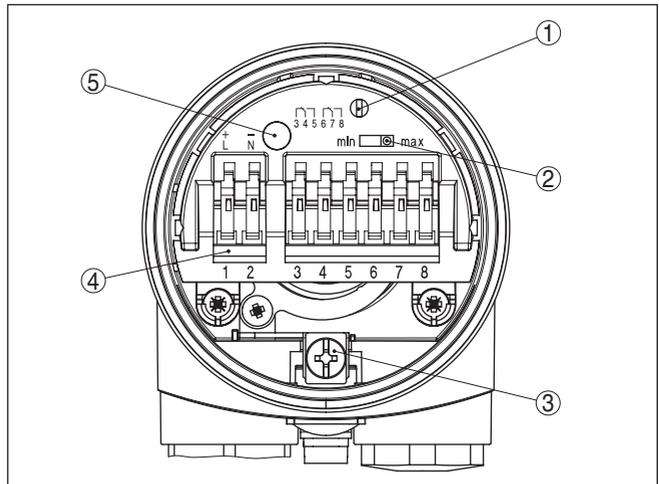
Fig. 11: Electronics and connection compartment - relay output
