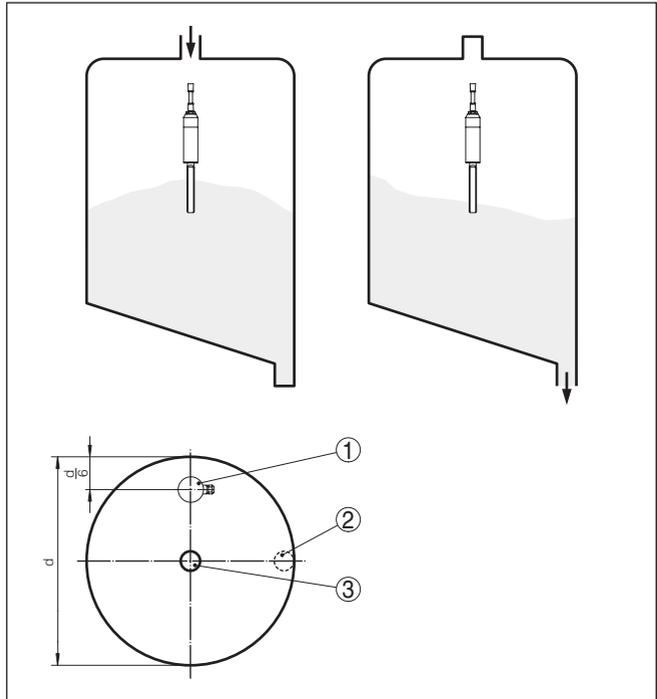
Fig. 4: Filling in the centre, emptying laterally
