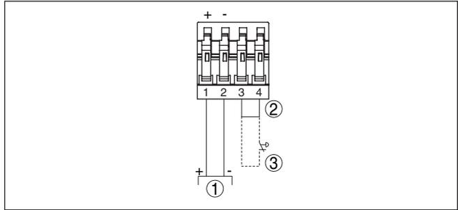
Fig. 11: Wiring plan - External simulation key
