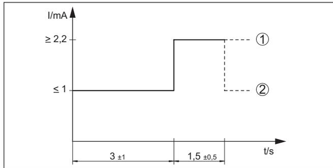
Fig. 14: Flow chart of the function test
