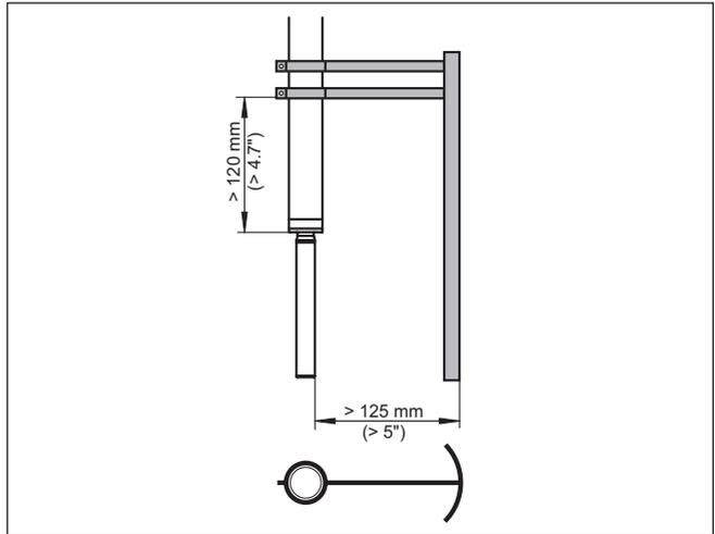
Fig. 7: Baffle for protection against mechanical damage
