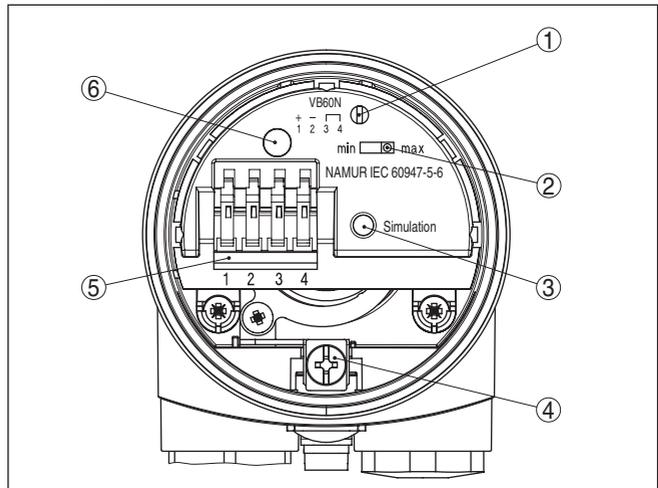
Fig. 13: Electronics and connection compartment - NAMUR output
