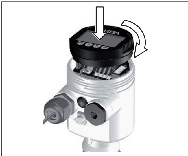
Fig. 26: Insert display and adjustment module
