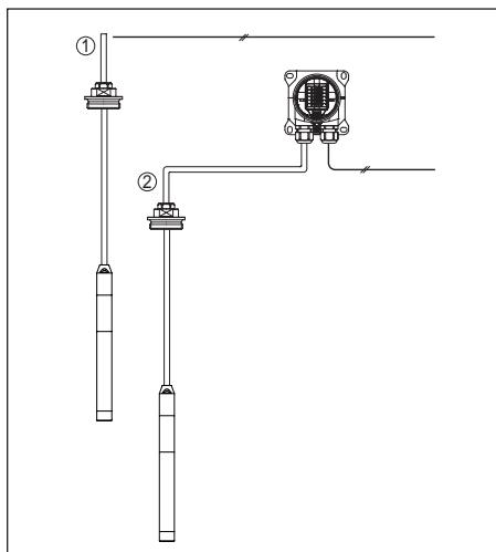
Abb. 15: Connect VEGAWELL S 51 to voltage supply
