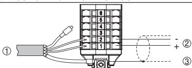
Abb. 17: Wiring plan VEGA WELL S 51 4 ... 20 mA, 4 ... 20 mA/HART
