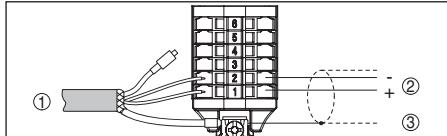
Abb. 26: Schéma de raccordement VEGA WELL S 51 4 ... 20 mA, 4 ... 20 mA/HART
