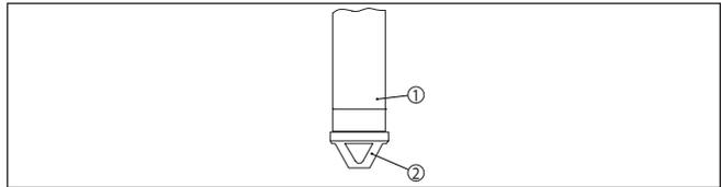
Fig. 4: VEGAWELL 52, transport and mounting protection
