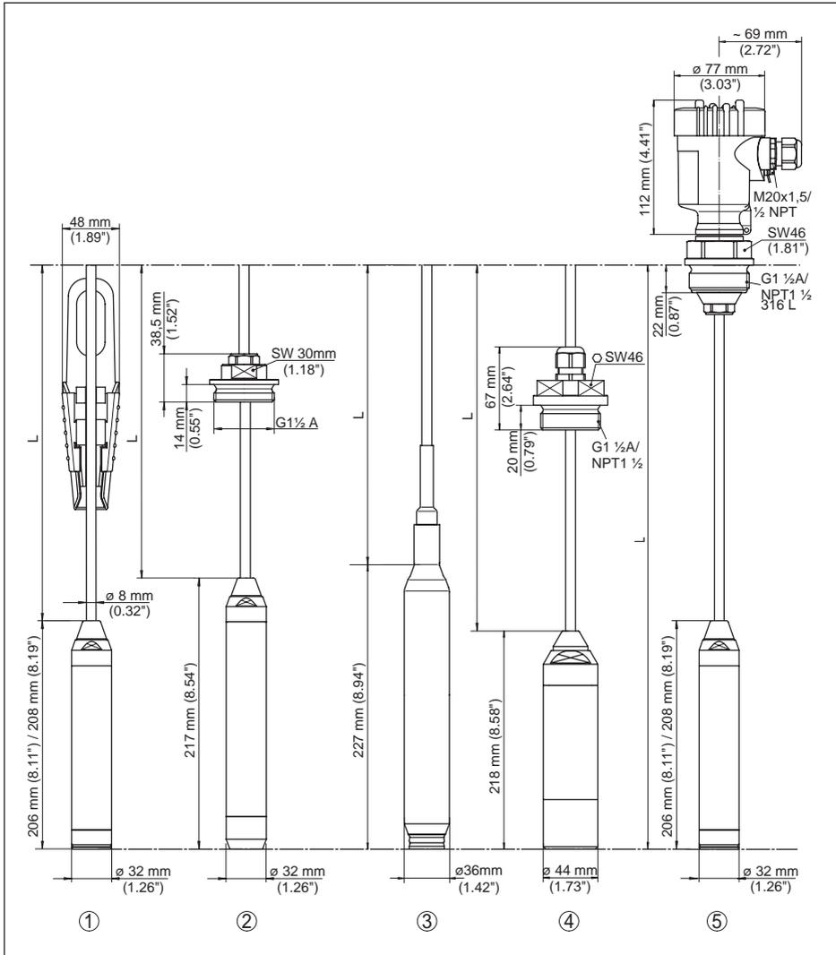
Fig. 18: VEGAWELL 52, with transmitter Duplex (1.4462)/PVDF
