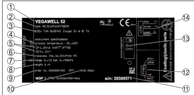
Fig. 2: Structure type label VEGAWELL 52 (example)
