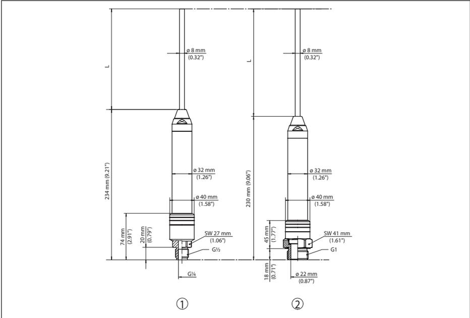
Fig. 19: VEGAWELL 52, with threaded fitting and transmitter Duplex (1.4462)
