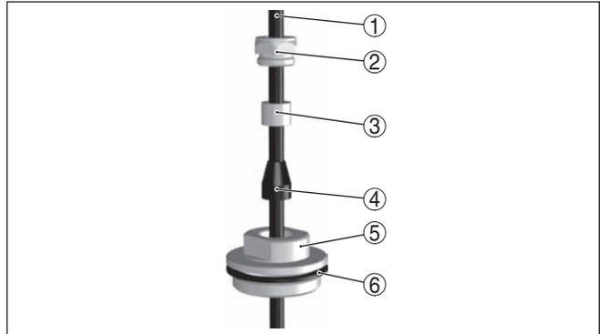
Fig. 7: Configuration, screw connection of suspension cable
