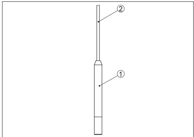
Fig. 1: Example of a VEGAWELL 52 with transmitter 22 mm
