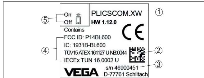
Fig. 1: Layout of the type label (example)
