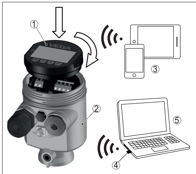
Fig. 2: Wireless connection to standard operating devices
