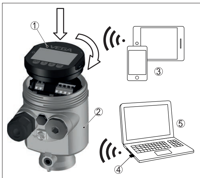
Fig. 2: Wireless connection to standard operating devices
