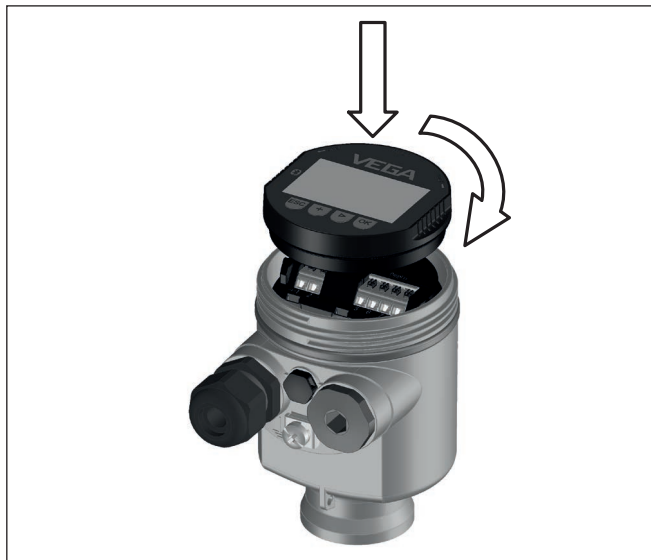
Fig. 29: Installing the display and adjustment module in the electronics compartment of the single chamber housing
