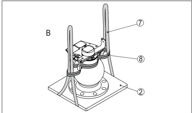
Fig. 12: Additional lug to prevent the source holder from tilting
