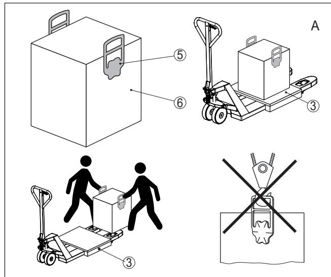
Fig. 10: Transport of the type A packaging
