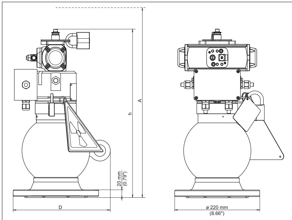
Fig. 51: Source holder VEGASOURCE 31, version K, L
