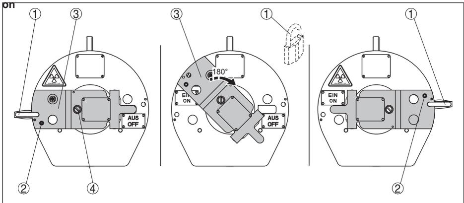
Fig. 33: Switching the radiation on - VEGASOURCE 31 version D
