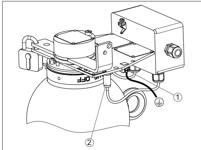
Fig. 28: Connection of the earth conductor terminal
