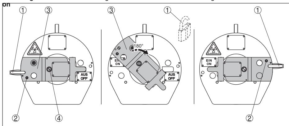
Fig. 33: Switching the radiation on - VEGASOURCE 31 version D
