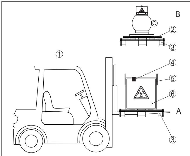
Fig. 11: Pallet transport of the type A packaging
