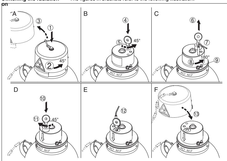
Fig. 30: Switching the radiation on - VEGASOURCE 31 version A
