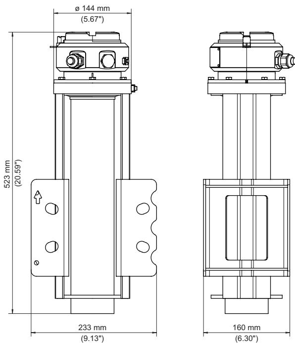
Fig. 55: Gamma modulator for uninterrupted measurement even with X-ray radiation
