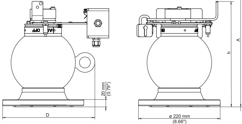
Fig. 50: Source holder VEGASOURCE 31, version E (stirrup for manual ON/OFF switching, padlock for securing the switch position ON or OFF, in addition with electrical position indicators)
