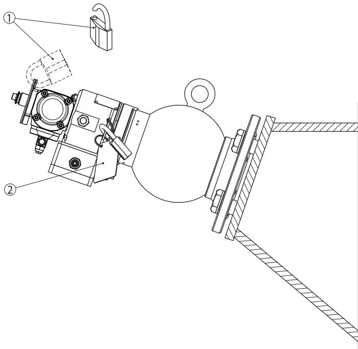
Fig. 34: Switching on the radiation with pneumatic switching facility - VEGASOURCE 31 version K, M
