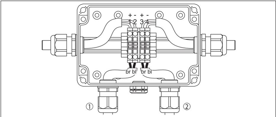
Fig. 29: Connection terminal housing of the position indicators
