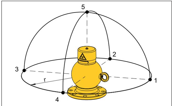
Fig. 36: Measuring points for the measurement of the local dose rate
