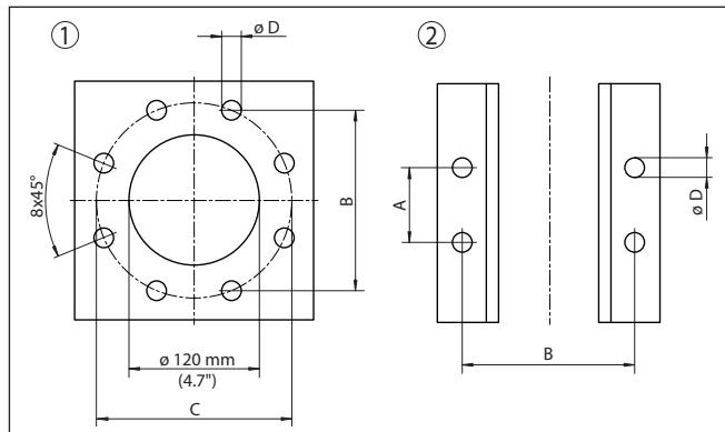
Fig. 25: Mounting facility supplied by the customer
