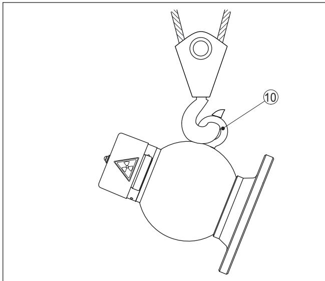
Fig. 13: Crane transport of the source holder
