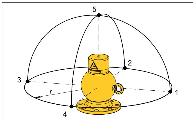
*Fig. 36: Measuring points for the measurement of the local dose rate*
