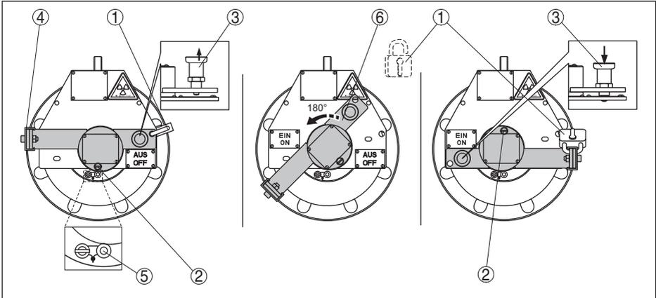
Fig. 31: Switching the radiation on - VEGASOURCE 31 version B
