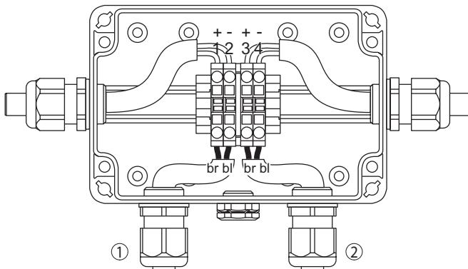
Fig. 26: Connection terminal housing of the proximity switches
