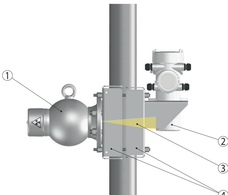
Fig. 57: Mounting brackets for mounting on pipes from 50 ... 220 mm (1.97 ... 8.66 in) for 30° diagonal irradiation
