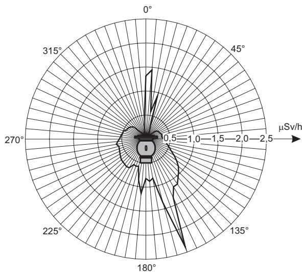
Fig. 45: Dose rate diagram (distance: 1 m) - example: source holder VEGASOURCE 31 with Cs-137, 100 mCi (3.7 GBq)
