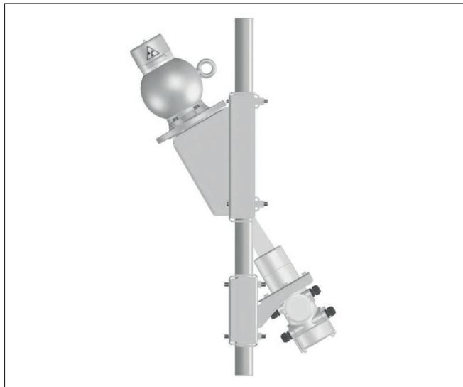
*Fig. 18: 30° measurement setup on a pipeline with diameter 50 ... 100 mm
