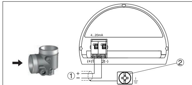
插图. 31: 防爆 (Ex-d-ia) 型双腔式壳体的接线腔
