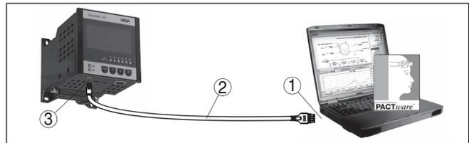
Fig. 7: Connection of the PC via USB
