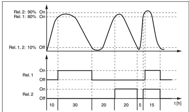
Fig. 10: Example of pump control 2
