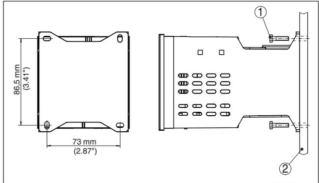
Fig. 3: Screw mounting
