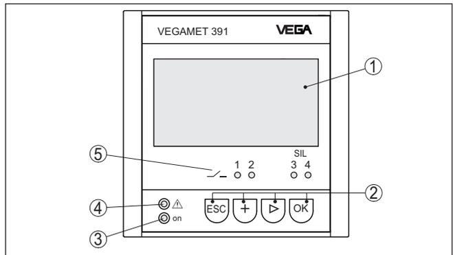
Fig. 6: Display and adjustment elements
