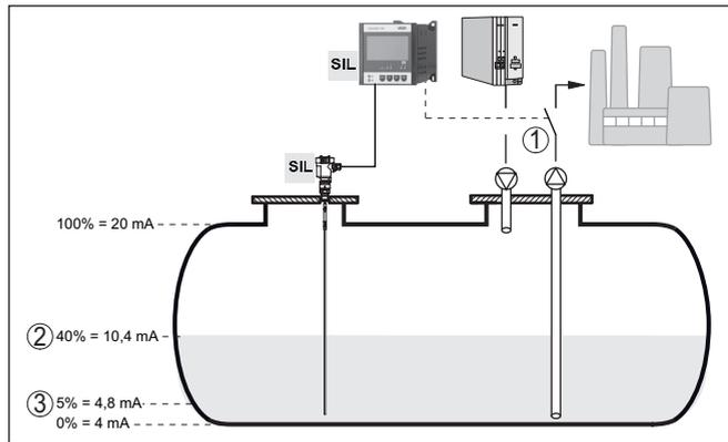
Fig. 9: Dry run protection according to SIL2
