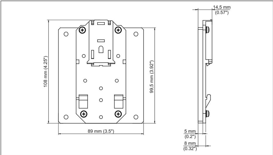
Fig. 12: Dimensions of optional carrier rail adapter
